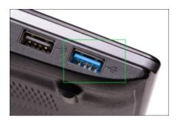
Confirm that you are using a SuperSpeed Cable; the regular speed cable will not work with the Intel Camera.
